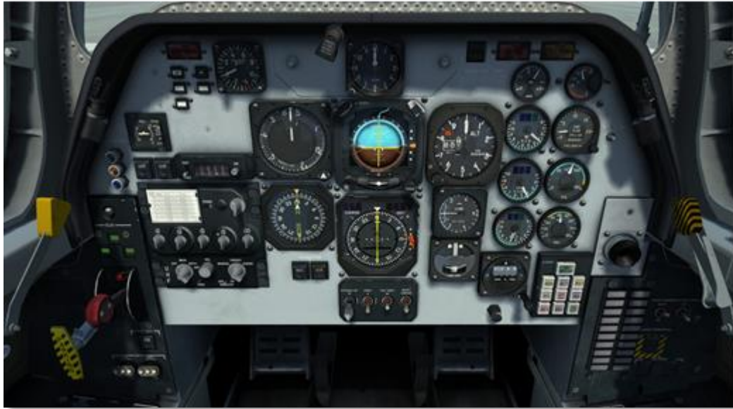
Figure 3-7 Rear main panel
