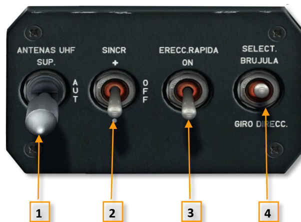
Figure 3-79 TARSYN control panel
