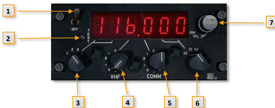
Figure 3-71 VHF radio panel
