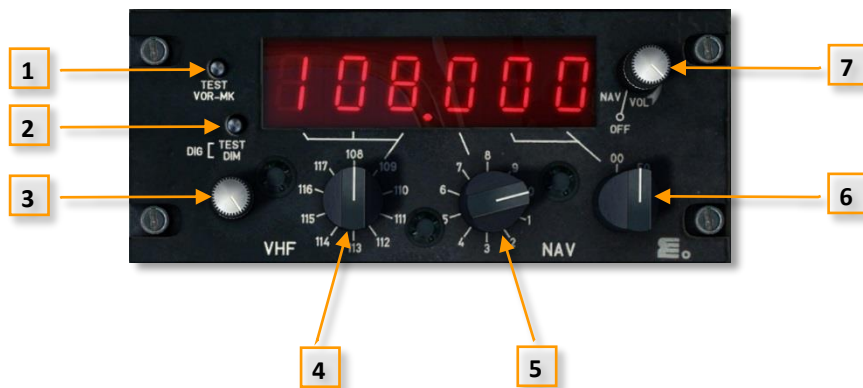
Figure 3-73 VOR/ILS control panel
