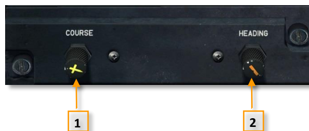
Figure 3-78 HSI remote control panel
