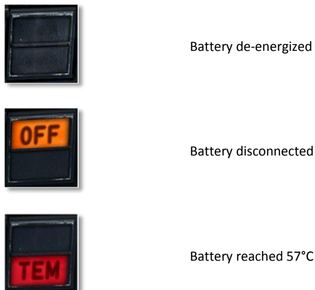
Figure 3-29 Battery isolation/warning switch
